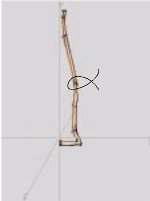
**51** Use the *Axis Move* command with the magnet option to move the point collection away from the Y axis along the X axis.
